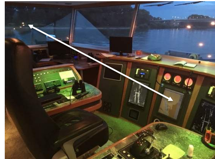
Figure 17. The distance from seat (eyes) to ECDIS (straight ahead/down) can be quite large in some vessels up to approx. 1,9m. Legibility of characters can be difficult.
