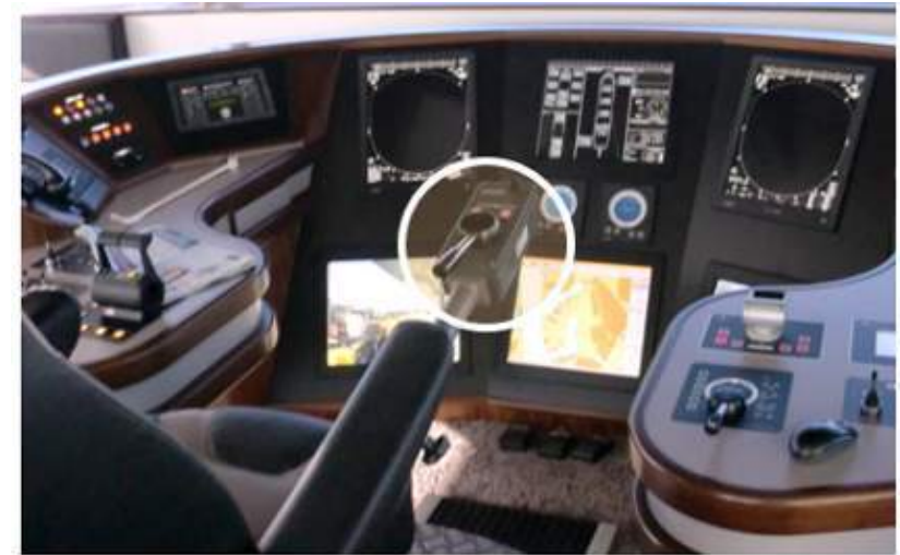
Figure 19. Example of a control on a pod mounted on the arm rest.
