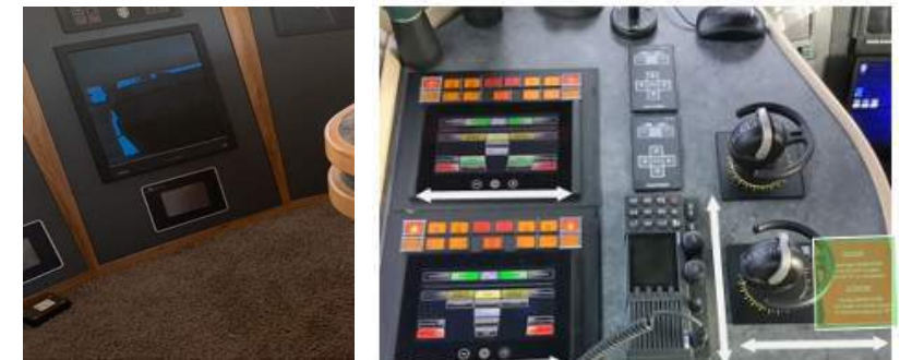
Figure 20: Left - Example of non-matted screen for radar or ECDIS, leading to impaired legibility
