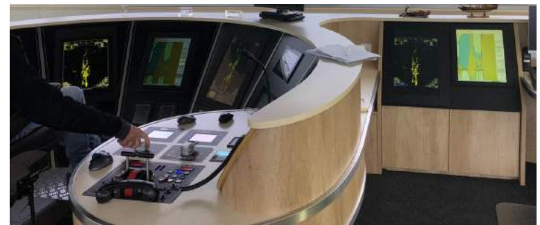
Figure 11. Example of an auxiliary workstation with ECDIS and Radar next to the helmsman's position to implement the coaching task, in this case combined with the administration and cargo planning task area.
