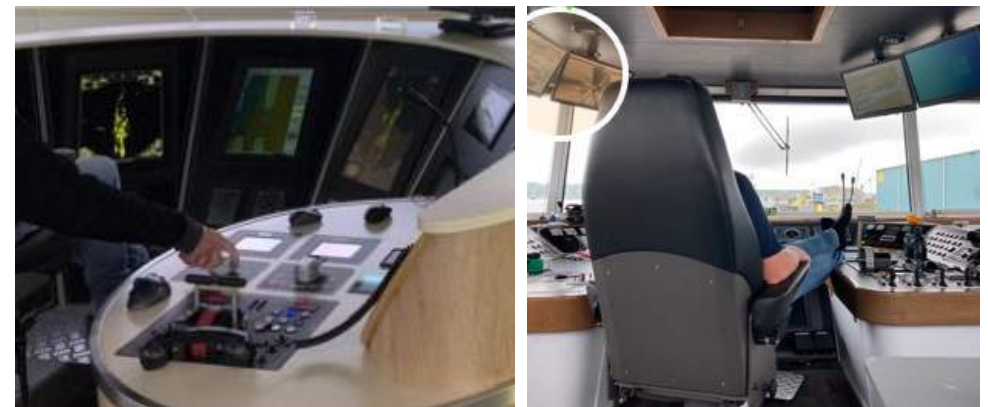
Figure 18. (Left) Engine control within reach but outside primary grasping area. (Right) Twisted leaning working position to compensate far reaching.
