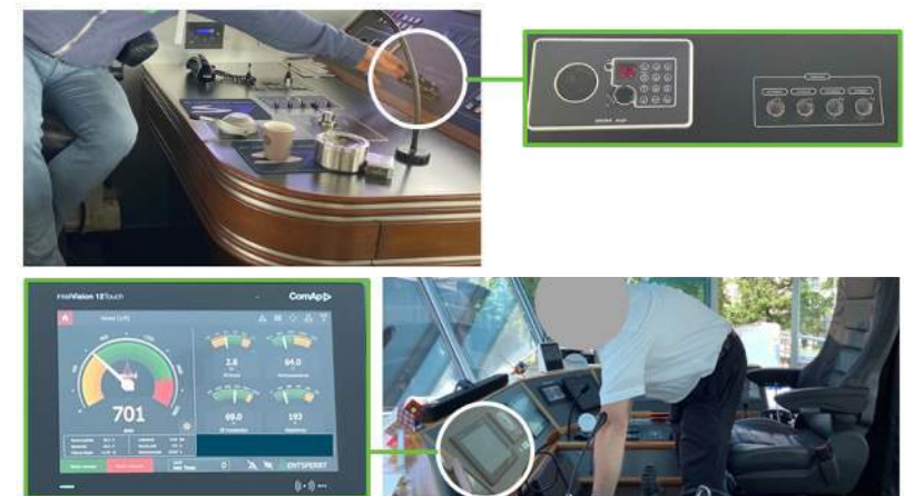
Figure 16. Observations from vessel visits: unfavourable working postures when operating VHF (top) and a motor management touchscreen (bottom).
